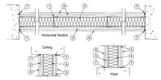
1. Studs — Channel-shaped, min 3-5/8 in. wide by 1-1/4 in. deep with 5/16 in. folded back return flange legs. Fabricated from No. 25 MSG galv steel. Max stud spacing 24 in. OC. Studs to be cut 3/4 in. less than assembly height.
