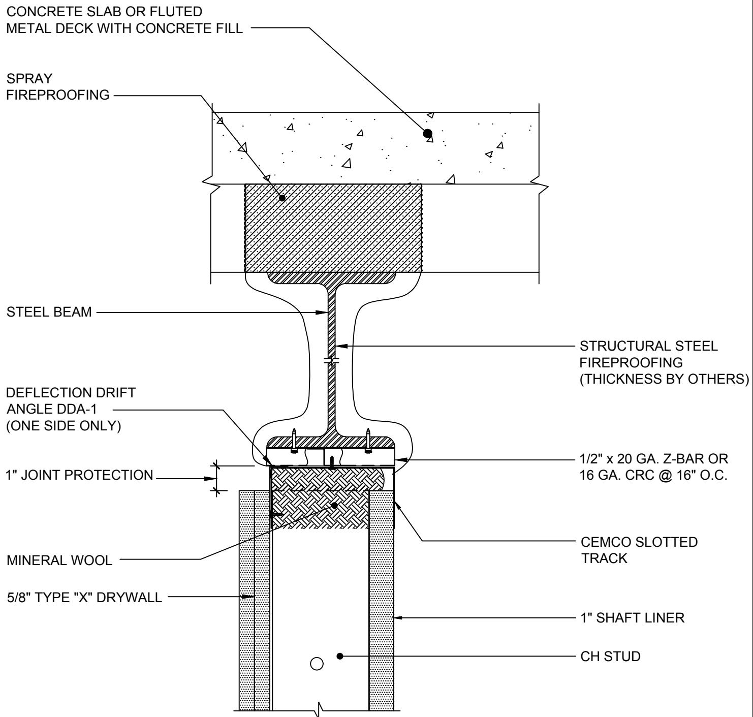
NOTE: SINGLE LAYER OF  $\frac{5}{8}$ " TYPE "X" DRYWALL FOR 1 HOUR FIRE RATING
