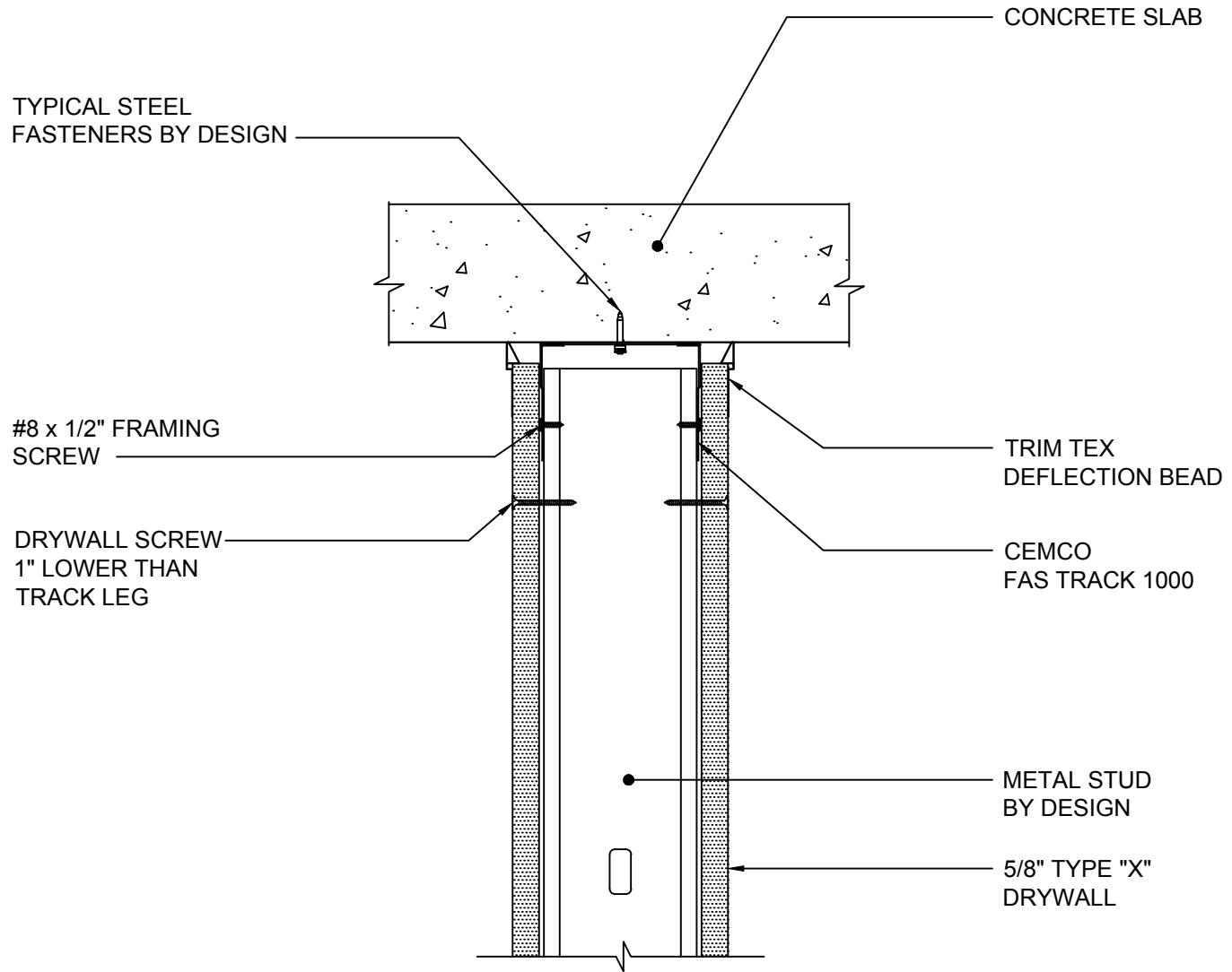
NOTE: DOUBLE LAYERS OF  $\frac{5}{8}$ " DRYWALL FOR 2 HOUR FIRE RATING
