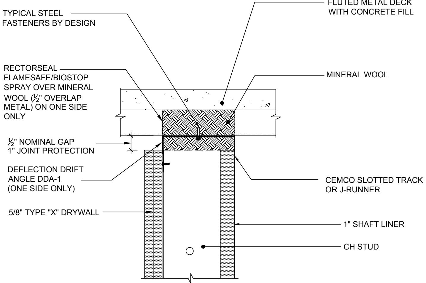
NOTE: SINGLE LAYER OF  $\frac{5}{8}$ " TYPE "X" DRYWALL FOR 1 HOUR FIRE RATING
