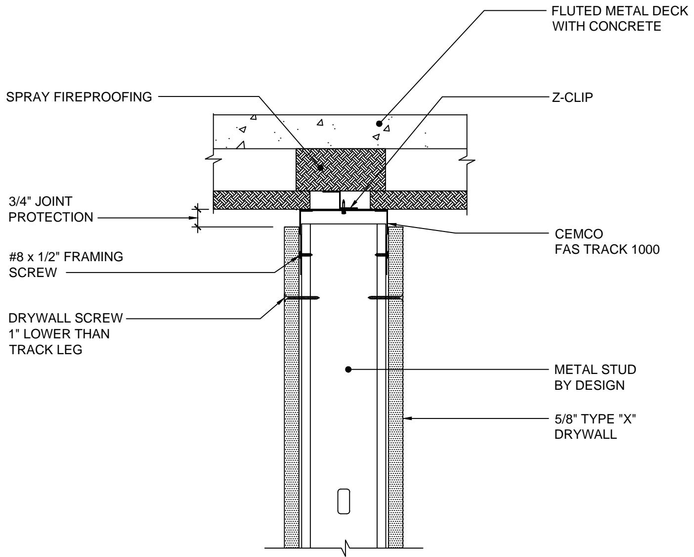
NOTE: DOUBLE LAYER OF  $\frac{5}{8}$ " TYPE "X" DRYWALL FOR 1 HOUR FIRE RATING
