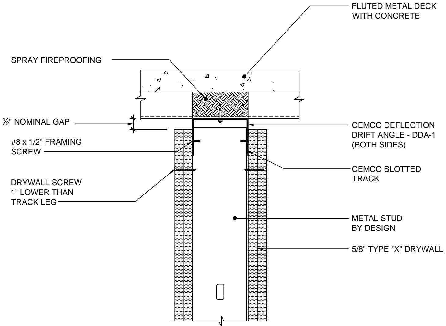
NOTE: SINGLE LAYER OF  $\frac{5}{8}$ " TYPE "X" DRYWALL FOR 1 HOUR FIRE RATING
