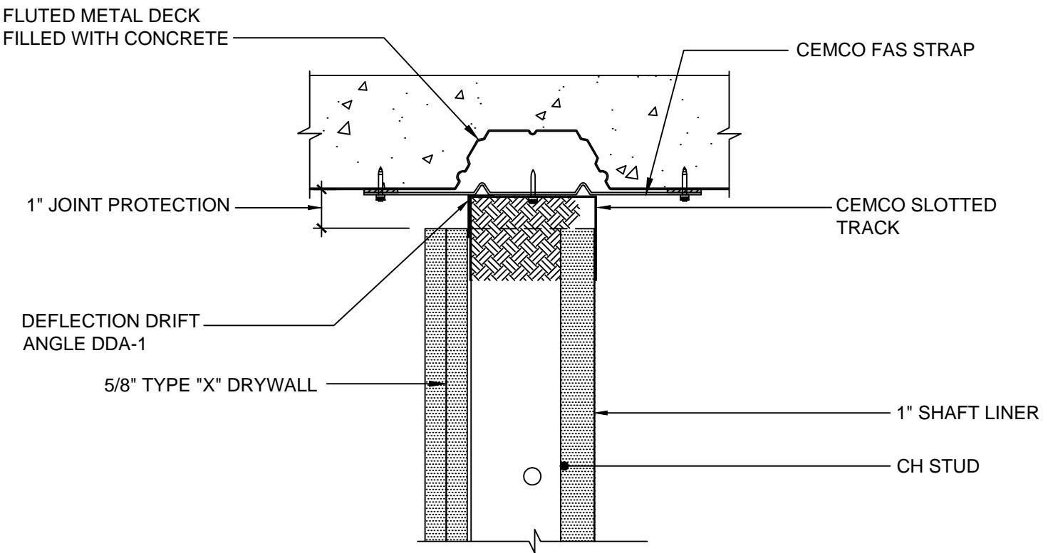
NOTE: SINGLE LAYER OF  $\frac{5}{8}$ " TYPE "X" DRYWALL FOR 1 HOUR FIRE RATING
