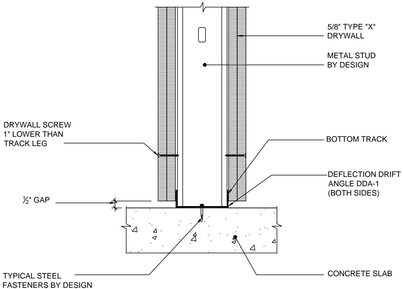
NOTE: SINGLE LAYER OF  $\frac{5}{8}$ " TYPE "X" DRYWALL FOR 1 HOUR FIRE RATING
