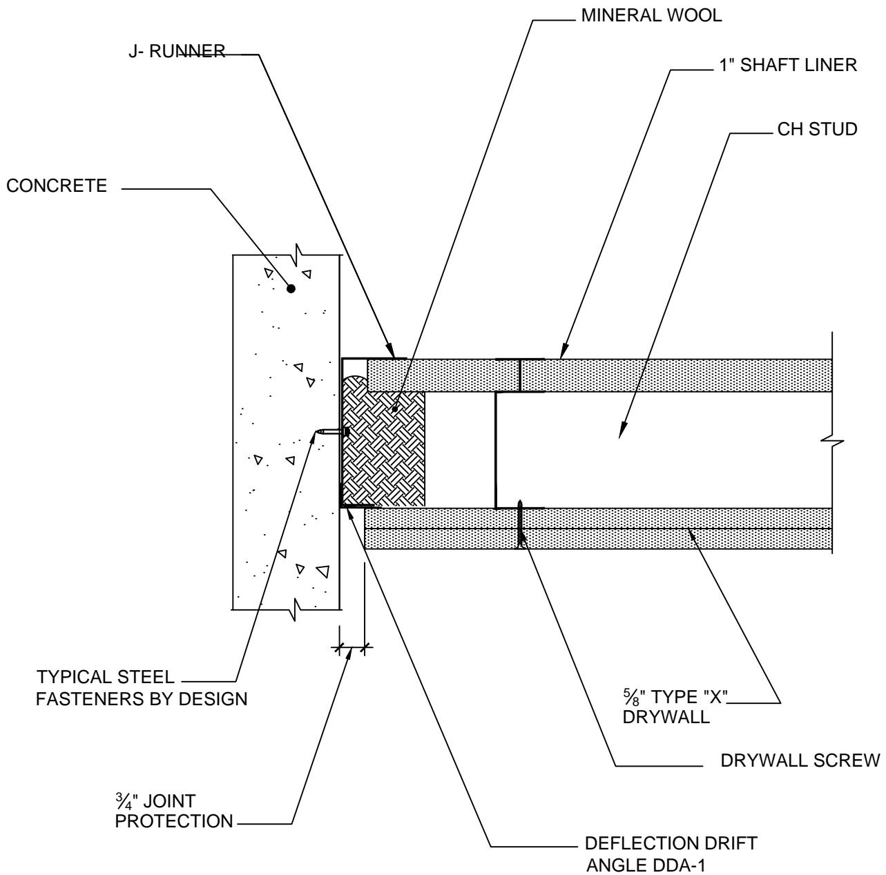
NOTE: SINGLE LAYER OF  $\frac{5}{8}$ " TYPE "X" DRYWALL FOR 1 HOUR FIRE RATING
