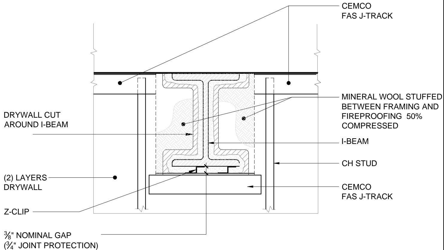
NOTE: SINGLE LAYER OF  $\frac{5}{8}$ " TYPE "X" DRYWALL FOR 1 HOUR FIRE RATING
