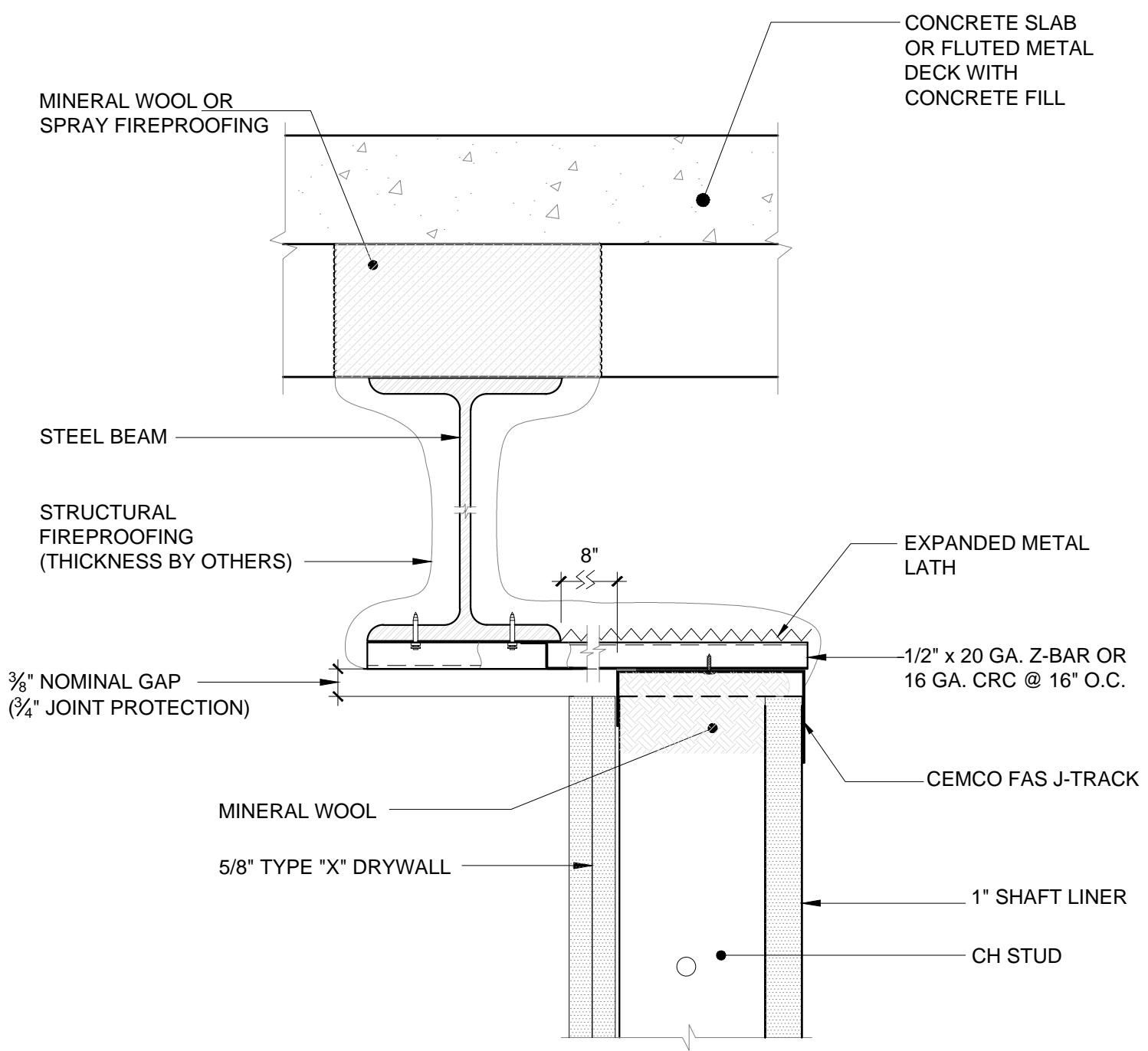
NOTE: SINGLE LAYER OF  $\frac{5}{8}$ " TYPE "X" DRYWALL FOR 1 HOUR FIRE RATING
