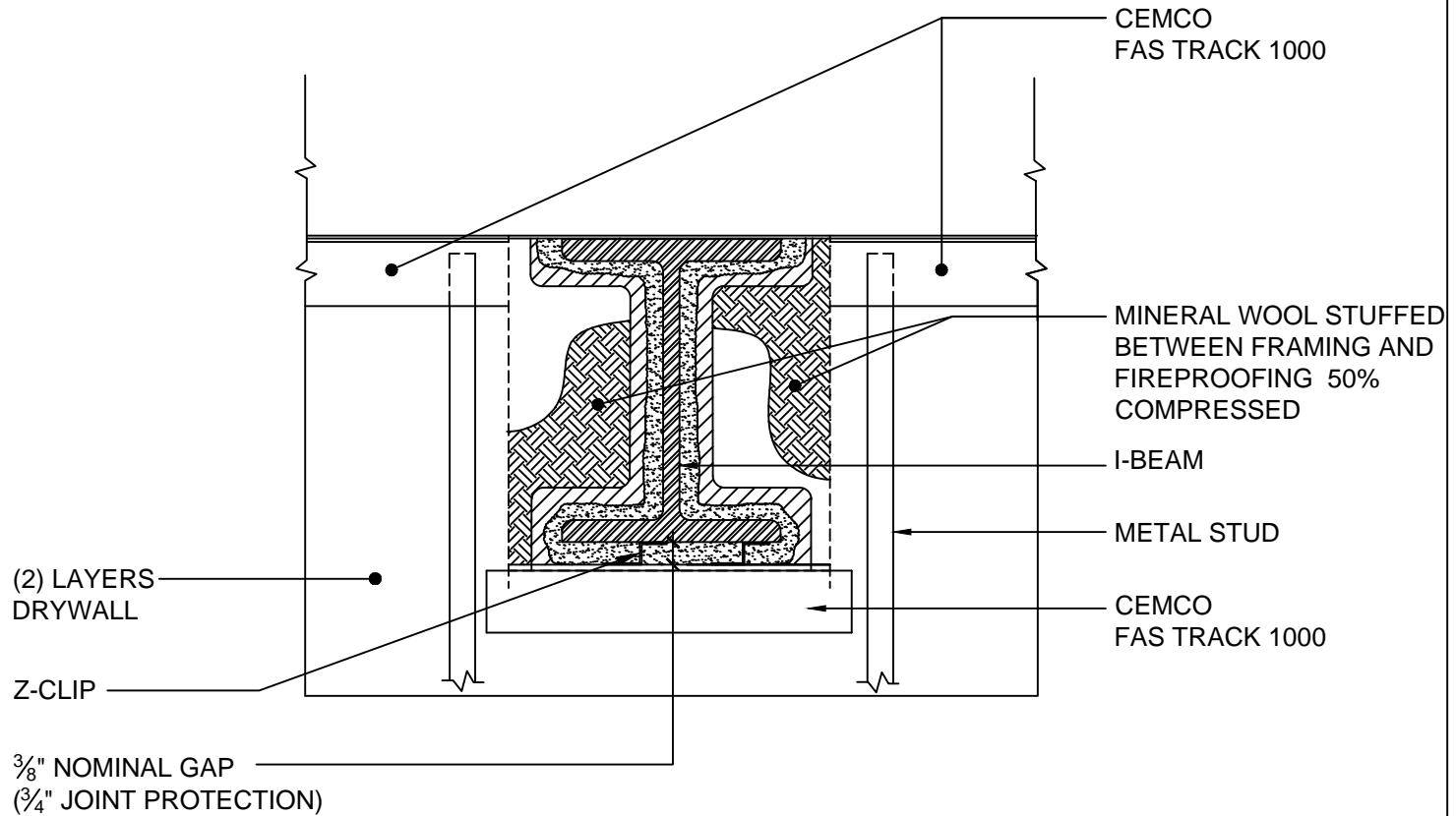
NOTE: SINGLE LAYER OF  $\frac{5}{8}$ " TYPE "X" DRYWALL FOR 1 HOUR FIRE RATING
