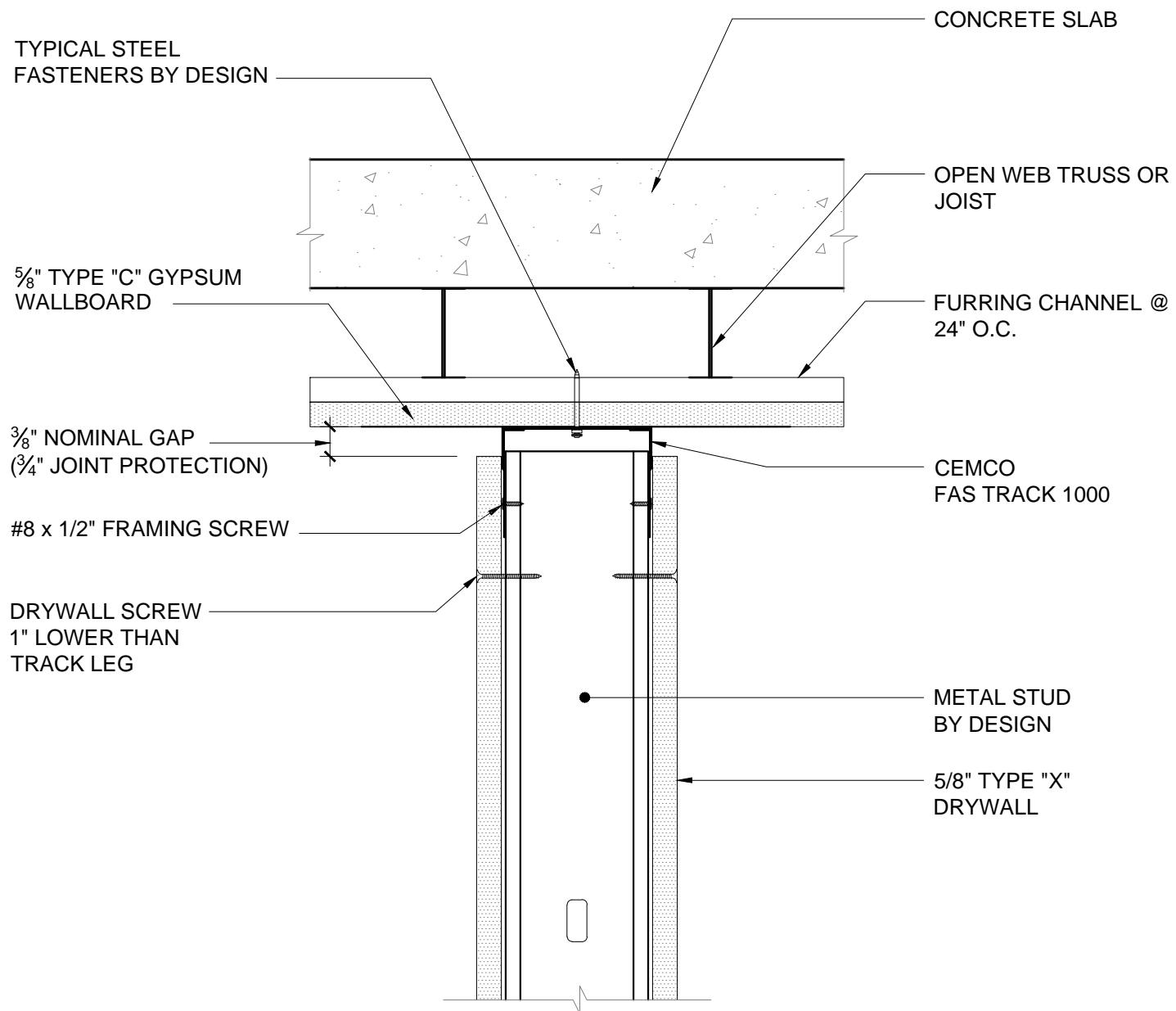
NOTE: SINGLE LAYER OF  $\frac{5}{8}$ " TYPE "X" DRYWALL FOR 1 HOUR FIRE RATING
