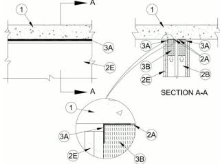
1. Floor Assembly — Min 4-1/2 in. (114 mm) thick steel-reinforced lightweight or normal weight (100-150 pcf or 1600-2400 kg/m²) structural concrete. Floor may also be constructed of any min 6 in. thick (152 mm) UL Classified hollow-core Precast Concrete Units\*.
