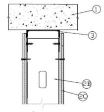
1. Floor Assembly — Min 4 1/2 in. (114 mm) thick steel reinforced lightweight or normal weight (100-150 pcf or 1600-2400 kg/m<sup>2</sup>) structural concrete. Floor may also be constructed of any min 6 in. thick UL Classified hollow-core **Precast Concrete Units\***. See **Precast Concrete Units\***.
