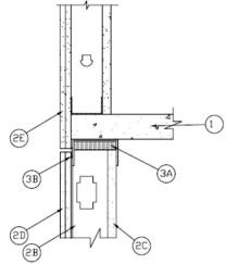
1. Floor Assembly — Min 4-1/2 in. (114 mm) thick steel reinforced lightweight or normal weight (100-150 pcf or 1600-2400 kg/m<sup>2</sup>) structural concrete. Floor may also be constructed of any min 6 in. (152 mm) thick UL Classified hollow-core **Precast Concrete Units\***. See **Precast Concrete Units** (CFTV) category in the Fire Resistance Directory for names manufacturers.
