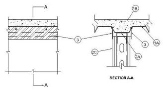
bly — The fire-rated fluted steel deck/concrete floor assembly shall be constructed of the materials and in the manner described in the individual D700 or D900 Series Floor-Ceiling Design in the UL Fire Resistance Directory and shall include the following construction
