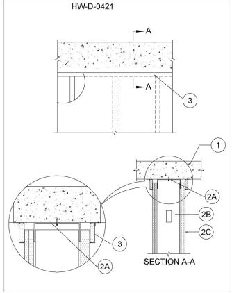
1. Floor Assembly — Min 4-1/2 in. (114 mm) thick steel reinforced lightweight or normal weight (100-150 pcf or 1600-2400 kg/m<sup>2</sup>) structural concrete. Floor may also be constructed of any min 6 in. thick UL Classified hollow-core **Precast Concrete Units\***. See **Precast Concrete Units** (CFTV) category in the Fire Resistance Directory for names of manufacturers.
