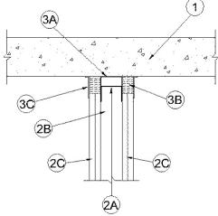
1. Floor Assembly — Min 4-1/2 in. (114 mm) thick steel reinforced lightweight or normal weight (100-150 pcf or 1600-2400 kg/m<sup>3</sup>) structural concrete. Floor may also be constructed of any min 6 in. (152 mm) thick UL Classified hollow-core **Precast Concrete Units\***. See **Precast Concrete Units** (CFTV) category in the Fire Resistance Directory for names of manufacturers.
