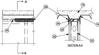
1. Floor Assembly — The fire-rated fluted steel deck/concrete floor assembly shall be constructed of the materials and in the manner described in the individual D700 or D900 Series Floor-Ceiling Design in the UL Fire Resistance Directory and shall include the following construction
