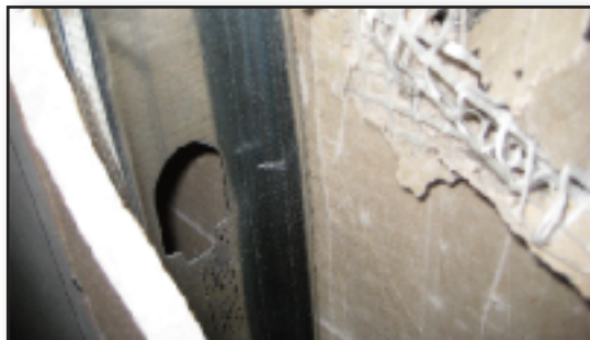
Soft body impact test using ViperStud.
