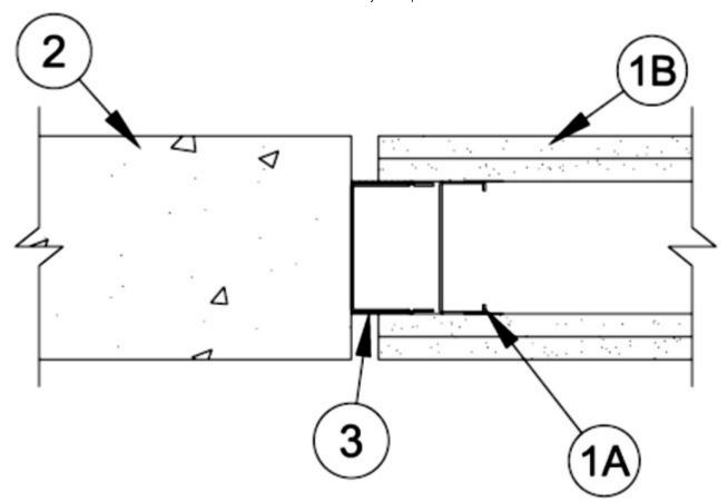
1. **Wall Assembly** — The 1 or 2 hr fire-rated gypsum board/steel stud wall assembly shall be constructed of the materials and in the manner described in the individual U400 or V400 Series Wall and Partition Design in the UL Fire Resistance Directory and shall include the following construction features:
