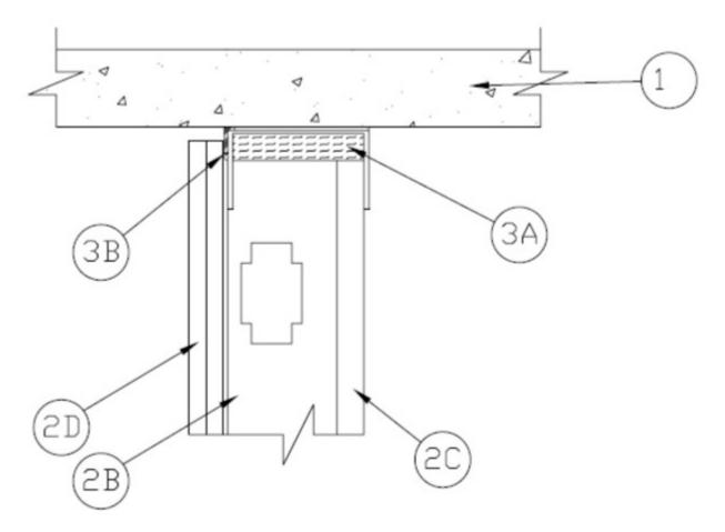
1. **Floor Assembly** — Min 4-1/2 in. (114 mm) thick steel reinforced lightweight or normal weight (100-150 pcf or 1600-2400 kg/m<sup>3</sup>) structural concrete. Floor may also be constructed of any min 6 in. thick UL Classified hollow-core Precast Concrete Units\*.
