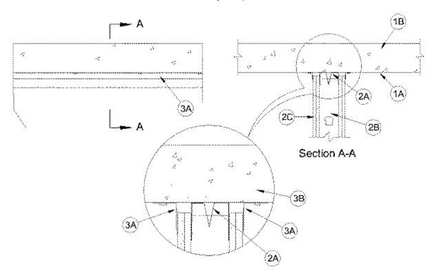
1. **Floor Assembly** — Min 4-1/2 in. (114 mm) thick steel reinforced lightweight or normal weight (100-150 pcf or 1600-2400 kg/m<sup>3</sup>) structural concrete. Floor may also be constructed of any min 6 in. thick UL Classified hollow-core **Precast Concrete Units\***.
