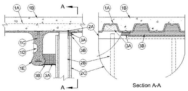
1. **Floor Assembly** — The fire-rated fluted steel deck/concrete floor assembly shall be constructed of the materials and in the manner described in the individual D700 or D900 Series Floor-Ceiling Design in the UL Fire Resistance Directory. The hourly
