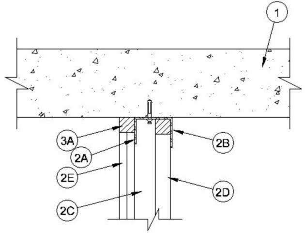
1. **Floor Assembly** — Min 2-1/2 in. (64 mm) thick reinforced lightweight or normal weight (100-150 pcf or 1600-2400 kg/m<sup>3</sup>) structural concrete. Floor may also be constructed of any 6 in. (152 mm) thick UL Classified hollow-core Precast Concrete Units\*.
