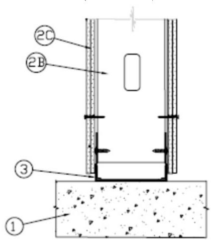
1. **Floor Assembly** — Min 4 1/2 in. (114 mm) thick steel reinforced lightweight or normal weight (100-150 pcf or 1600-2400 kg/m³) structural concrete. Floor may also be constructed of any min 6 in. thick UL Classified hollow-core **Precast Concrete Units\***.
