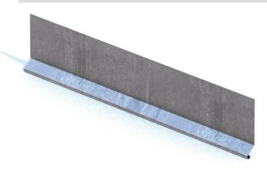
The #12 SOFFIT DRIP EDGE is manufactured for soffit and recessed windows head application. The 45° slope allows water to weep out of the assembly. The Drip edge provides a place for water to drip from rather than travel back along the soffit. The #12 SOFFIT DRIP EDGE fabricated from minimum 0.018-inch thick hot dipped galvanized steel having a minimum G-90 coating.
