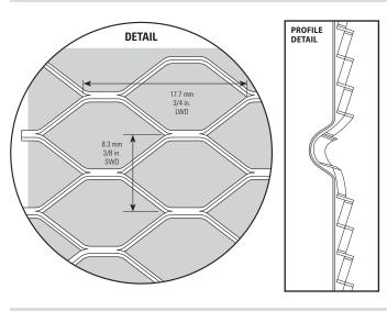
CEMCO's Self Furred Diamond Metal Lath "Dimpled" is available with Grade D asphalt paper backing. A saturated black asphalt paper complying with Federal Spec. No. UUB-790A Style 2 Grade D. Manufactured with a 3" lap for weathered application. CEMCO Self-Furring Dimpled with D-paper metal lath is produced from standard G60 hot-dipped galvanized steel. G90 is available upon special request. 25 bundles per pallet.
