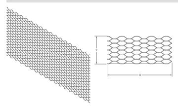
Stripite product is a general purpose expanded metal lath for plaster reinforcement. Stripite is a perfect addition to doors, windows, and other areas where cracking will most likely occur. Stripite is also used as a grout stop in cement block construction. Stripite is manufactured from 2.5 lath in standard G60 hot-dipped galvanized steel. G90 is available upon special request.
