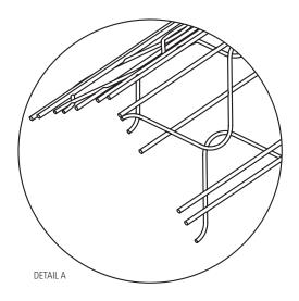
CEMCORNER is used as an exterior corner reinforcement that has a nailing strip along both sides for faster installation and straighter corners. CEMCORNER was designed so that it is easier for Portland cement plaster to flow into the nose of the CEMCORNER. CEMCORNER is fabricated from 17.5 GA. [0.054 inch diameter] galvanized welded-wire. CEMCORNER is available in the following configurations:
