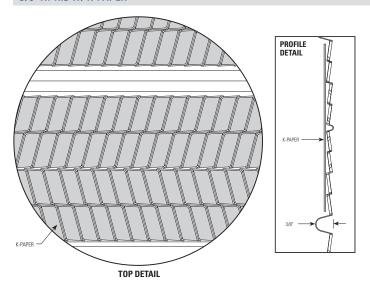
CEMCO's 3/8" Hi-Rib Lath is available with 3" strips of K-Paper attached to the spaces between the 3/8" ribs to minimize blow through of plaster when machine applied. This lath can be used in both vertical and horizontal applications. CEMCO 3/8" Hi-Rib w/ K-Paper is fabricated from 0.015-inch-thick in standard G60 hot-dipped galvanized steel. G90 is available upon special request.
