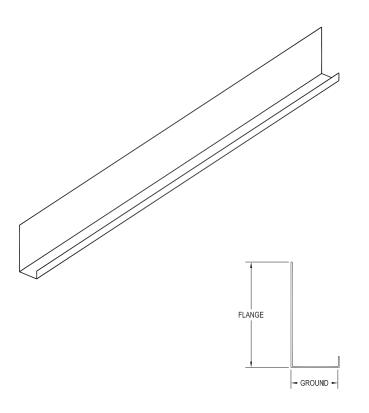
"J" Metal products are manufactured in various grounds (depths) to be used with a variety of polystyrene or foam insulation boards for exterior purposes. "J" Metal also provides for a workable screed around doors and windows. "J" Metal can also be ordered with holes and be used in some applications as a weep screed, and with a short flange (1-3/4") or long-flange (3-1/2"). CEMCO's J-Metal is fabricated from 26 ga., G60 hot-dipped galvanized steel. G90 coating is available upon request.
