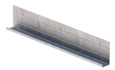
The J-SERIES CASING BEAD is manufactured non-perforated to enable the casing bead to have solid flashing capabilities. J-Series Casing Bead is fabricated from minimum 0.018-inch thick hot-dipped galvanized steel having a minimum G-90 coating.
