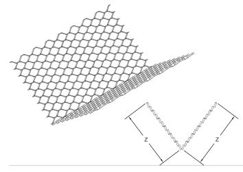
Cornerite is a smooth edge expanded metal lath corner reinforcement formed at a 105° angle to ensure a snug fit. This product also easily flattens for general patching. Cornerite is manufactured from steel meeting 0.016" thickness. Cornerite is manufactured from 1.75 expanded metal lath in standard G60 hot-dipped galvanized steel. G90 is available upon request.
