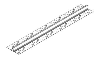
CEMCO's FAS-093X Fire Rated control joint is a composite control joint with intumescent tape factory applied to the back side of the control joint. The opening is protected by an orange plastic tape to indicate the fire rating. This tape is removed after joint compound has been applied and the finish is completed. The section is fabricated from standard G40 hot-dipped galvanized steel.
