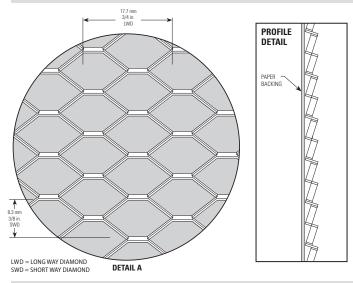
CEMCO's Diamond Metal Lath is available with Grade D asphalt paper backing. A saturated black asphalt paper complying with Federal Spec. No. UUB-790A Style 2 Grade D. Manufactured with a 3" lap for weathered application. All CEMCO expanded metal lath is produced from standard G60 hot-dipped galvanized steel. G90 is available upon special request. 25 bundles per pallet.
