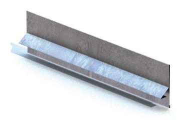
The #7 EXTENDED FOUNDATION SCREED provides an additional layer of 25 ga. G90 metal to protect waterproof deck membranes at the base wall from U.V. degradation. The #7 EXTENDED FOUNDATION SCREED is fabricated from minimum 0.018-inch thick hot-dipped galvanized steel having a minimum G-90 coating.
