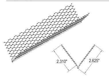
1-A Expanded Cornerbead is manufactured with 2-5/8" expanded metal flanges and a solid metal nose to provide for clean and sharp corners even over slightly irregular surfaces. CEMCO's No. 1-A Expanded Metal Cornerbead is manufactured by Niles and distributed by CEMCO. No. 1-A Cornerbead is fabricated from 26 Gauge galvanized steel with G60 coating. G90 coating is available upon request.
