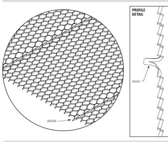
CEMCO's Self Furred Diamond Metal Lath "Grooved" is manufactured with 5 "V"-grooves in the lath in lieu of standard "dimples." These 5 grooves provide the necessary ¼" furring off the sheathing's surface to allow for proper embedment and keying of the scratch coat on all types of walls. CEMCO Self-Furring Grooved metal lath is produced from standard G60 hot-dipped galvanized steel. G90 is available upon special request. 50 bundles per pallet.
