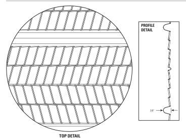
CEMCO's 3/8" Hi-Rib Lath is the most rigid of all metal laths. With full 3/8" ribs longitudinally spaced at 4" apart between each 3/8" rib with a 1/8" rib. Hi-Rib lath is able to span up to 24" on center. This lath can be used in both vertical and horizontal applications. Please consult CEMCO's Technical Services for specifics. CEMCO 3/8" Hi Rib lath is fabricated from 0.015-inch-thick in standard G60 hot-dipped galvanized steel. G90 is available upon special request.
