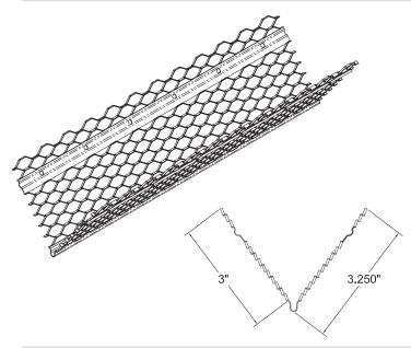
2-A Expanded Cornerbead is manufactured with extra long 3-1/4" flanges and a reinforced steel rib running the entire length of the piece to provide for extra rigidity when nailing to the corner. CEMCO's 2-A Cornerbead is manufactured by Niles Inc. No. 2-A Cornerbead is fabricated from 26 Gauge galvanized steel with G60 coating. G90 coating is available upon request.
