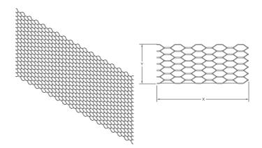
Patches are a recent development by CEMCO based on a timeless use of 2.5 diamond lath, but manufactured in strips or 'patches' to be used over door and window corners to greatly reduce cracking, by reinforcing stress areas. Patches can also be used as grout stop in masonry applications. Patches is manufactured in standard G60 hot-dipped galvanized steel. G90 is available upon special request.
