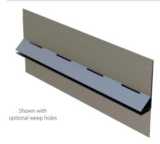
The M-SLIDE EXPANSION JOINT is manufactured for application where movement is anticipated. The self-aligning two-piece design allows for 1-inch vertical movement while maintaining a watertight assembly for plaster walls. M-Slide expansion joint is fabricated from minimum 0.018-inch thick hot-dipped galvanized steel having a minimum G-90 coating. Available with or without weep holes.
