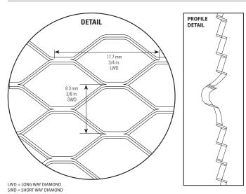
CEMCO's Self Furred Diamond Metal Lath "Dimpled" is manufactured with ¼" dimples in the lath. The dimples provide the necessary minimum ¼" furring off the sheathing's surface to allow for proper embedment and keying of the scratch coat on all types of walls. CEMCO Self-Furring Dimpled metal lath is produced from standard G60 hot-dipped galvanized steel. G90 is available upon special request. 50 bundles per pallet.
