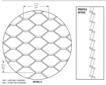
CEMCO's Diamond Metal Lath is a versatile base for cement plaster walls. Its carefully formed diamond keys allow for proper embedment and keying of the scratch coat on all types of walls. Can be used with hand and machine applied plaster. All CEMCO expanded metal lath is produced from standard G60 hot-dipped galvanized steel. G90 is available upon special request. 50 bundles per pallet.
