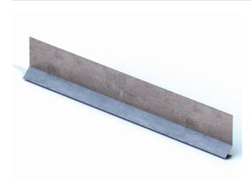
The #6 HEAD DRIP SCREED is manufactured for application above windows, doors, base of walls, and vents on exterior plaster walls. The 45° slope allows water to weep out of the assembly, and the 90° return provides a 3/4-inch solid metal leg for sealant application from stucco assembly to dissimilar materials. #6 Head/Foundation Drip Screed is fabricated from minimum 0.018-inch thick hot-dipped galvanized steel having a minimum G-90 coating.
