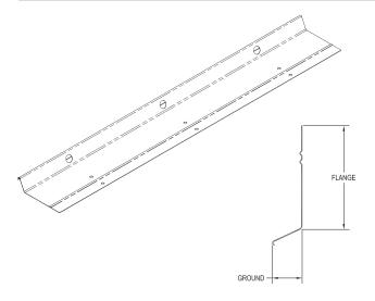
CEMCO's #36 Foundation Sill Screed is manufactured in 7/8" ground WITH 1/2" weep holes for drainage. The lack of a full-return on the bottom allowing for trowel access to clean access stucco material, leaving no visible metal below the stucco finish line. No. 36 sill screed is fabricated from 26 ga., G60 hot-dipped galvanized steel. G90 coating is available upon request.
