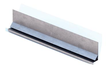
The #3 FLASHING SCREED is manufactured for applications above windows, doors and vents on exterior plaster walls. The #3 Flashing Screed consists of a combined single piece 45° weep screed, for drainage, an a Z flashing for window head protection. Available with or without weep holes. The #3 Flashing Screed is fabricated from minimum 0.018-inch thick hot-dipped galvanized steel having a minimum G-90 coating.
