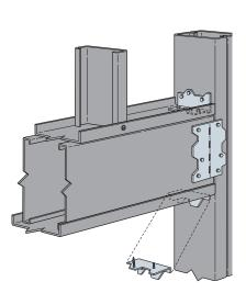
Typical Installation for Gravity Headers
