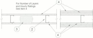
1. Floor and Ceiling Runners — (Not Shown) — For Use with Item 2 — Channel shaped, fabricated from min 25 MSG corrosion-protected steel, min depth as shown in item 4, attached to floor and ceiling with fasteners 24 in. OC max.
