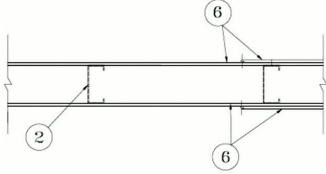
1. Floor and Ceiling Runners — (Not Shown — For the 1/2 or 1 Hour Nonbearing Wall Ratings) — For use with Item 2 - Channel shaped, fabricated from min 25 MSG corrosion-protected steel, min depth to accommodate stud size, with min 1-1/4 in. long legs, attached to floor and ceiling with fasteners 24 in. OC max
