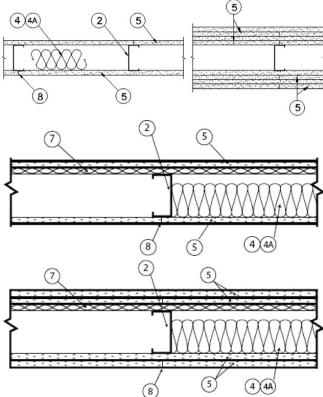
1. Floor and Ceiling Runners — (Not Shown) — Channel shaped, fabricated from min 25 MSG (0.018 in. min. bare metal thickness) corrosion-protected steel, min width to accommodate stud size, with min 1-1/4 in. long legs, attached to floor and ceiling with fasteners 24 in. OC max.
