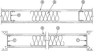
1. Floor and Ceiling Runners — Channel-shaped runners, min 2-1/2 in. wide by 1 in. deep, fabricated from 25 MSG galv steel. Attached to floor and ceiling with fasteners
