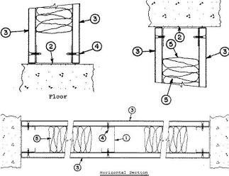
1. Studs — Channel-shaped, min 3-5/8 in. wide with 1-1/4 in. flanges and 3/8 in. lips. Fabricated from No. 25 MSG galv steel. Max stud spacing is 24 in. OC. Stud length cut 3/4 in. less than assembly height.
