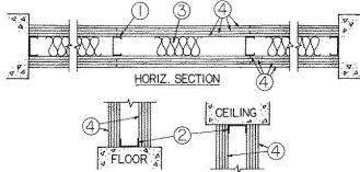
1. Studs — Channel-shaped, min 1-5/8 in. wide by 1 1/4 in. deep, with 5/16 in. folded back return flange legs. Fabricated from No. 25 MSG galv steel. Stud spacing 16 or 24 in. OC. Studs to be cut 1 in. less than assembly height.
