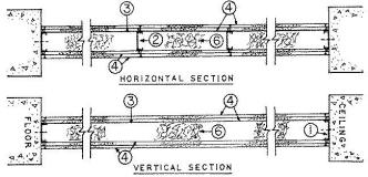
1. Floor and Ceiling Runners — Channel shaped 1/2 in. deep by min 3-5/8 in. wide, No. 25 gauge painted or galvanized steel. Min. No. 18 MSG for the 4 hour rating. Secured with 3/4 in. long concrete fasteners spaced 18 in. OC. For the 1 hour rating, width may be reduced to 2-1/2 in. to
