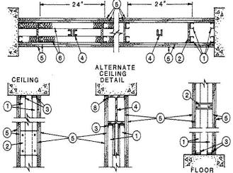
1. Studs — Channel-shaped, 1-5/8 in. wide by 1 in. deep, with 1/4 in. folded back return flange legs. Fabricated from No. 25 MSG galv steel. Studs spaced max 24 in. OC. Studs to be cut
