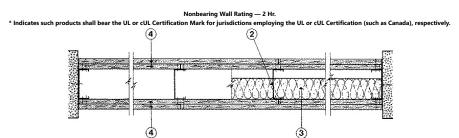
1. Floor and Ceiling Runner — (Not Shown) — Min. 25 MSG galv steel, 1 in, return legs, 2-1/2 in, deep (min), attached to floor and ceiling with fasteners 24 in, OC max.
