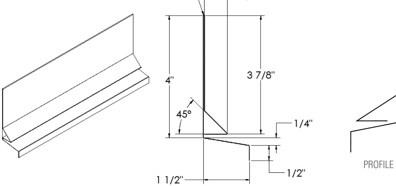
The **#3 FLASHING SCREED** is manufactured for applications above windows, doors and vents on exterior plaster walls. The #3 Flashing Screed consists of a combined single piece 45° weep screed, for drainage, an a Z flashing for window head protection. Available with or without weep holes.
